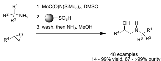
Scheme 22. Polymer-supported purification after aminolysis of oxiranes.
